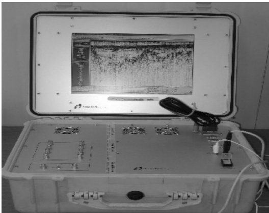
Fig. 3. The developed recording system.
