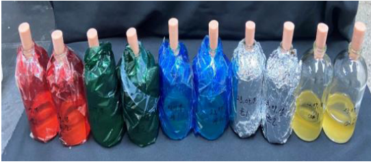
Fig. 1. Experimental setup adjusted to allow the penetration of light at different wavelengths.
