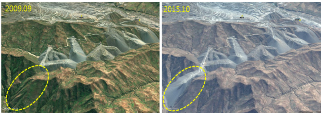
Fig. 3. The expansion of mine waste rocks from 2009 to 2015.
