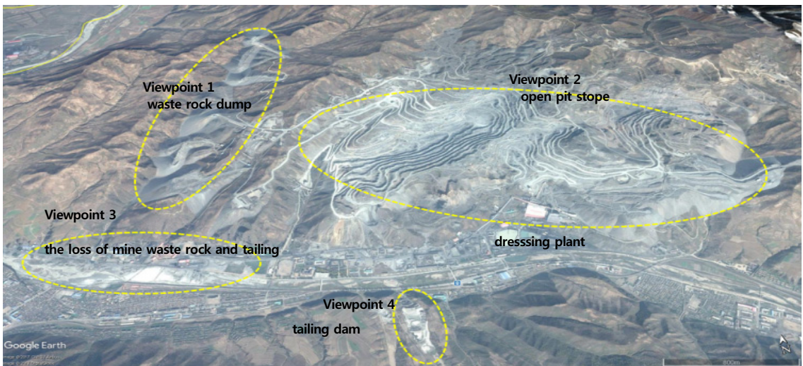
Fig. 2. The sites of mine hazards in Musan iron mine (2014).
