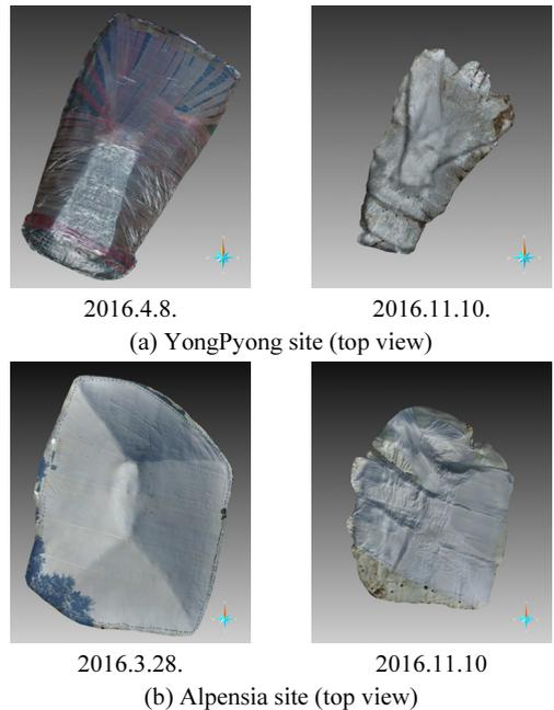
Fig. 7. Reconstructed 3D geometry model showing volume changes of snow stockpile during the storage period.
