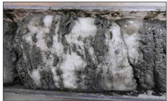
Fig. 9. Nodular gas hydrate sample recovered from Central Joetsu Basin (Matsumoto et al. , 2017).
