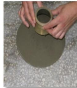
Fig. 4. Flow cone test.
