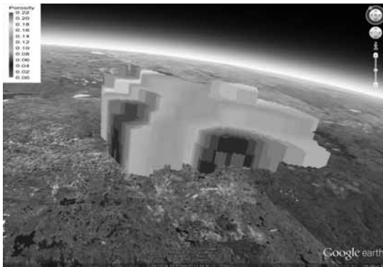
Fig. 7. Visualization of the 3D grid model representing the porosity distributions of Grosmont formation on Google Earth.
