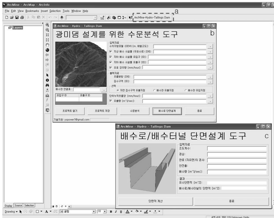
Fig. 6. Graphical user interface of the software developed in this study. (a) ArcMap extension toolbar. (b) Hydrological analysis tool. (c) Hydraulic design tool.
